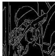
Figure 3.7. Result of SISO system with Canny edge detection.
